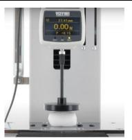
This unit is suitable for characteristic evaluation of such as cushioning-materials or press-fitted parts by compression test since it allows drawing a force-displacement graph and evaluating transition of the force value to the compressed displacement. Also, as you see in the picture above, it enables you to easily search for the force value at a specific displacement value on the graph and leave a comment.
