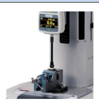
For example, in click sensation test of tactile switch, hysteresis and returning zero is obvious from the graph of a reciprocating motion. It is simple to evaluate the graph by setting threshold value, searching for returning peak values and inserting an arbitrary border line. Moreover, the point of switch ON/OFF can be automatically defined and displayed by using Mark On function.
