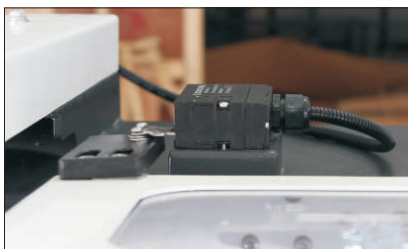
Door Safety Interlock system
