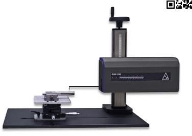
The PGS100 profilometer allows to acquire 2D profiles in an extremely simple and intuitive way, thanks also to its measuring range of 130 mm in length (X) and 50 mm in height (Z).
