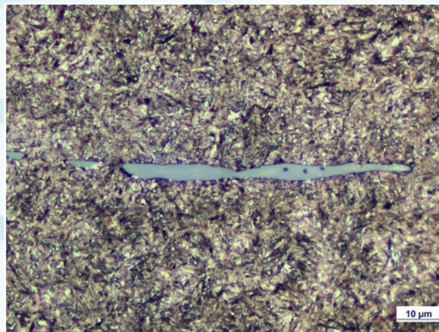
Tool Steel 100MnCrW4+QT, 700 HV, longitudinal section etched with Nital 3%, BF, 1000x
