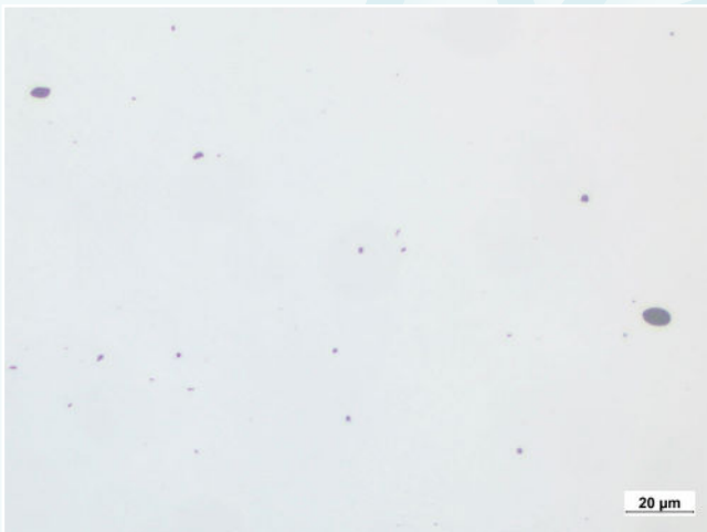
Low Alloy Steel 42CrMo4+QT, 330 HV, BF, 500x
