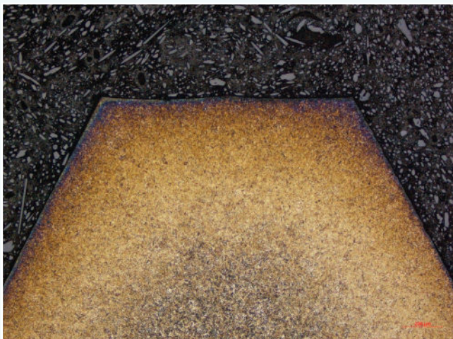
Etched with Nital 3%, BF, 50x
