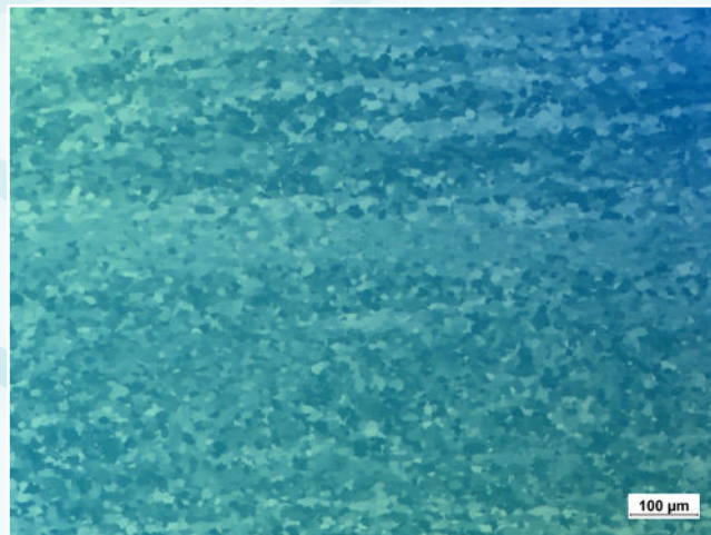
Pure Titanium, Grade 2, POL + Lambda Compensator, 100x
