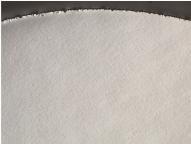
Pure Titanium, Grade 4, DIC, 100x
