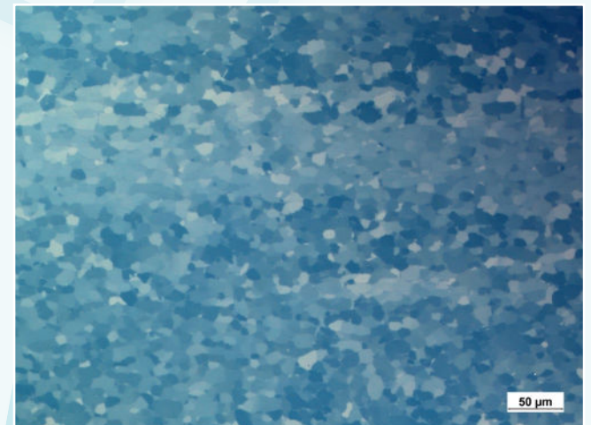
Pure Titanium, Grade 2, POL + Lambda Compensator, 200x
