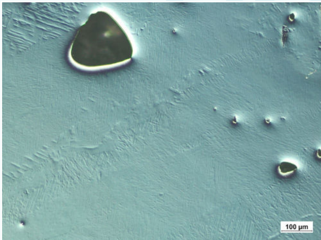
Ti6Al4V, Additive Manufacturing, DIC, 100x
